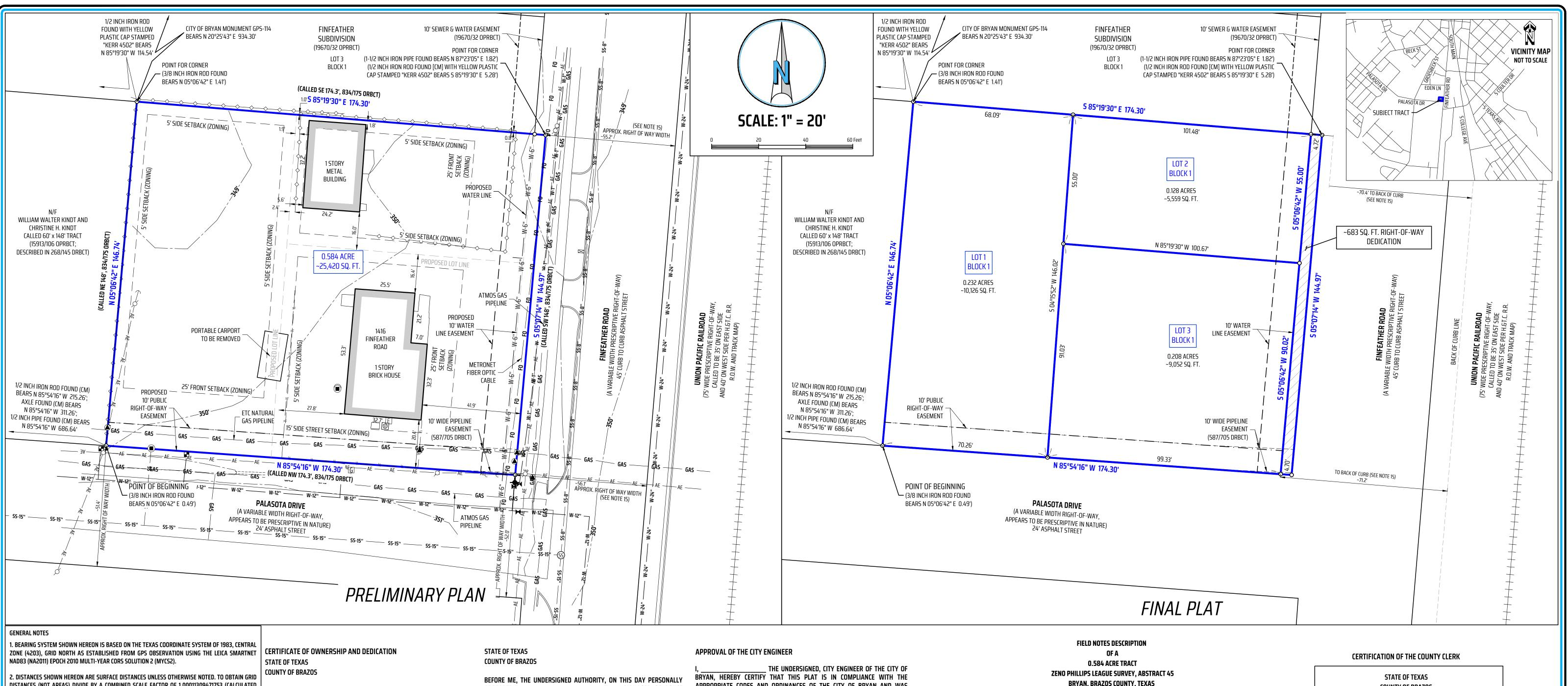
DISTANCES (NOT AREAS) DIVIDE BY A COMBINED SCALE FACTOR OF 1.00011309471753 (CALCULATED USING GEOID12B).
